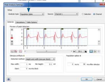
Above: Peak Analysis View displaying a spike. Left: Settings dialog with Detector (displayed), Calculations and Table Options tabs.
