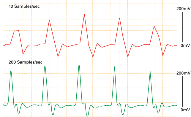
Figure 2A Undersampling - human finger pulse recorded at 10/s and 200/s. The former sampling rate is too low to depict the signal accurately.
