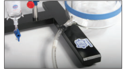
Connecting to Reservoir’s inlet
