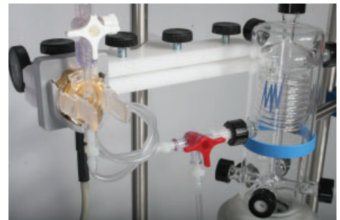
Connecting to the inlet of Perfusion Core via tubing
