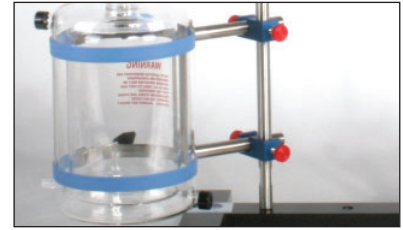
Attaching the other assembled Water Jacketed Reservoir on the left Support Rod
